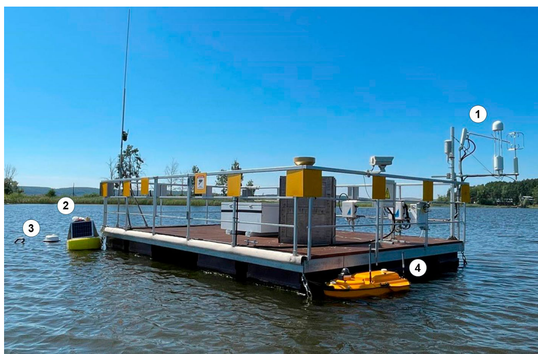
Fig. 7. Equipment complex at the Volga Carbon Supersite (aquatic site): 1—EC system on a stationary anchored pontoon; 2—ABS; 3—FC; 4—Apache USV.
