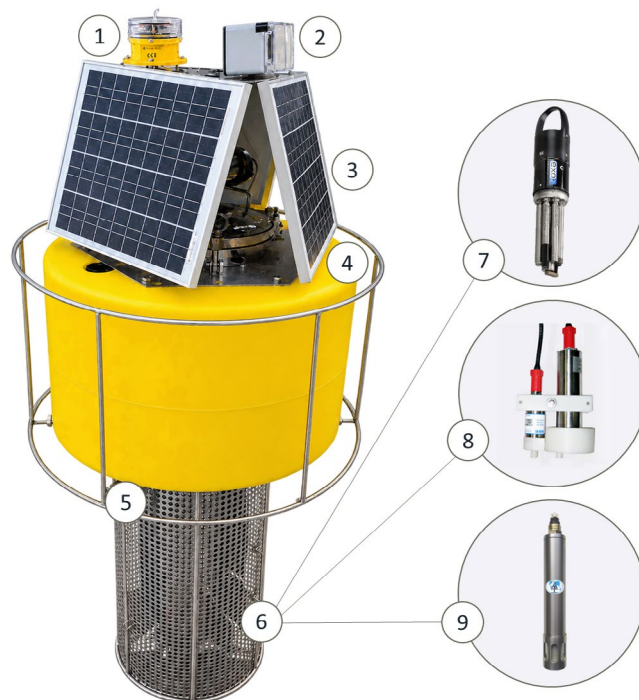
Fig. 2. ABS schematic: 1–beacon; 2–control/transmission module; 3–solar panels; 4–buoyancy hull; 5–protective frame; 6–sensor housing; 7–EXO2s sonde; 8–METS sensor (with SBE 5M pump); 9–AMT sensor.
