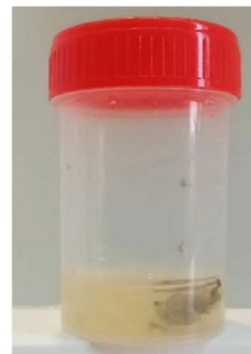
Fig.1. The appearance of the mycelium-like mass forming in aqueous dispersions of PVC nanoparticles at 10-11°C (PVC concentration is 328 mg/L, diameter of particle is 96 nm).
