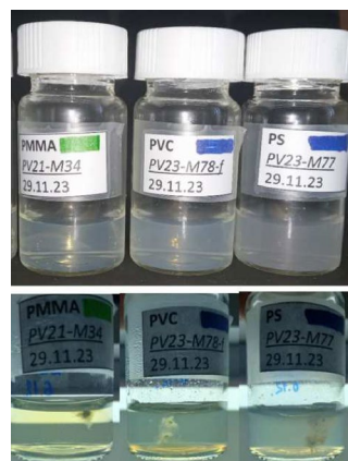
Fig.4. Photographs of synthetic polymer dispersions before (top) and after (bottom) inoculation with the L. coprophilum fungus and incubation for 76 days at 10–11°C. The initial nanoparticle concentration is 100 mg/L.
